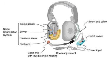
Figure 17.22 Headphones designed to cancel noise with destructive interference create a sound wave exactly opposite to the incoming sound. These headphones can be more effective than the simple passive attenuation used in most ear protection. Such headphones were used on the record-setting, around the world nonstop flight of the Voyager aircraft to protect the pilots' hearing from engine noise.
